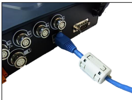
Installation of noise filter
